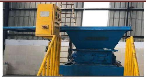
SHREDDER TO CUT WASTE AFTER AUTOCLAVING
