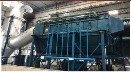
GAS COOLER (INDIRECT COOLING WITH WATER
