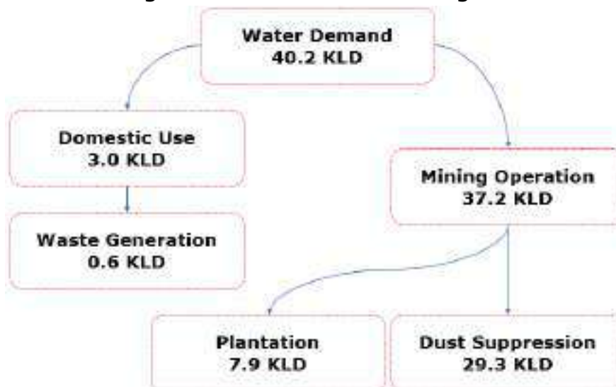
Figure 4.4: Water Balance Diagram
