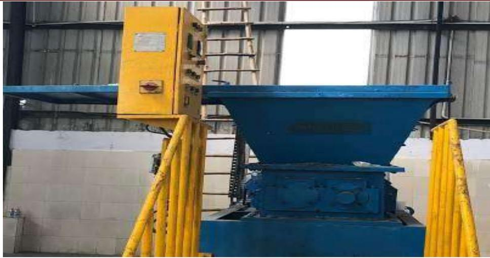
**SHREDDER TO CUT WASTE AFTER AUTOCLAVING**
