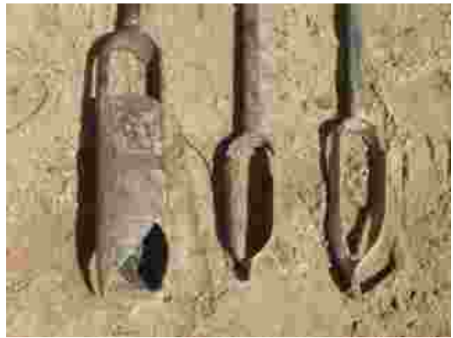
Figure III-2.2-iii.5b Example of augers. From left to right: Riverside (gravel, debris), auger (sand), Edelman auger
